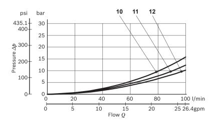
8 **(LF...)** | Stand alone 4/3, 4/2 solenoid operated directional valve Characteristic curves
