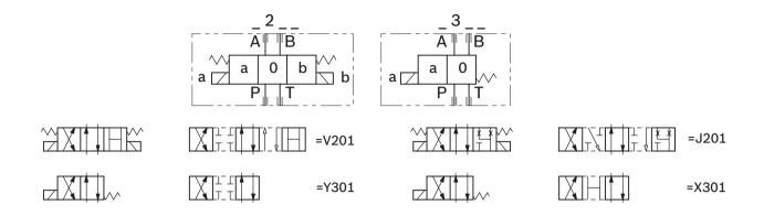
V201 for fixed displacement pumps - J201 for variable displacement pumps.
